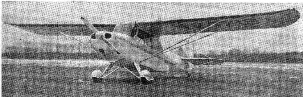
Standard equipment on the DeLuxe Traveler, on which most of our flight testing was done, includes a metal propeller with spinner, wheel pants, steerable tail wheel and navigation lights.
