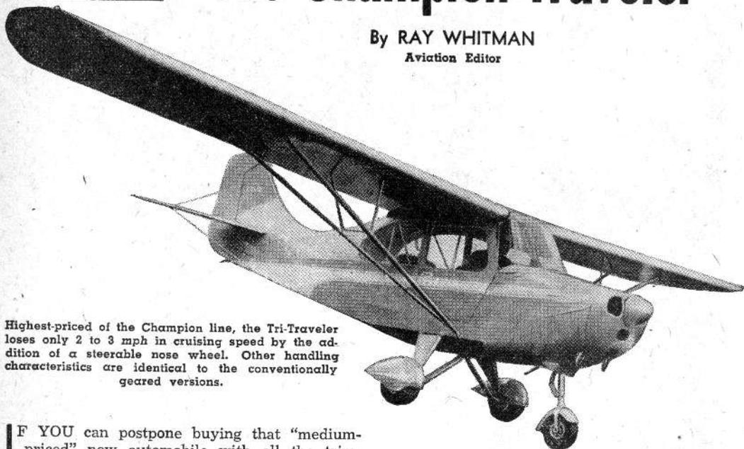
Highest-priced of the Champion line, the Tri-Traveler loses only 2 to 3 mph in cruising speed by the addition of a steerable nose wheel. Other handling characteristics are identical to the conventionally geared versions.
